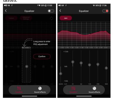
**Choose preset EQ:** swipe left or right on the bottom of the screen to switch equalizer.
